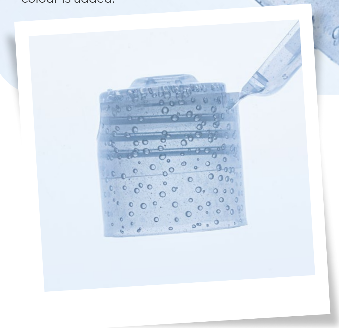
Close up showing bubbles evident in a plastic cap moulding. These are masked when colour is added.
